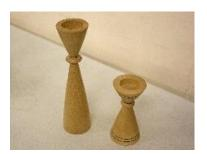
The piece was mounted between centres and a roughing gouge was used to produce a cylinder. A tenon was formed to fit the chuck and the piece was mounted in the chuck. Nikos then marked out the features with a pencil.
